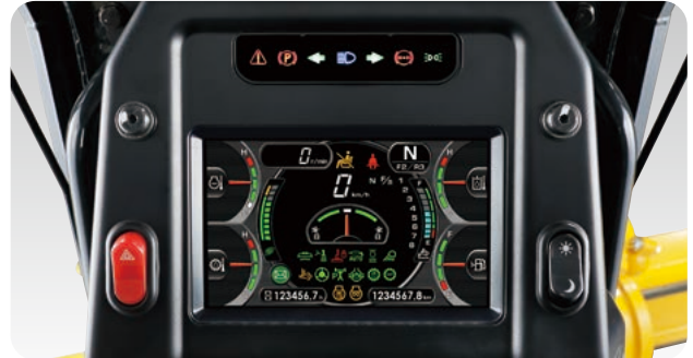
Photo is for Tier 4 Final machine. (DEF level gauge is only for Tier 4 Final machine.)
