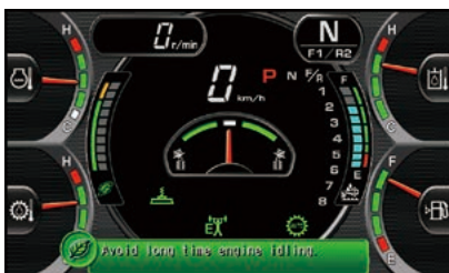
Photo is for Tier 4 Final machine. (DEF level gauge is only for Tier 4 Final machine.)
